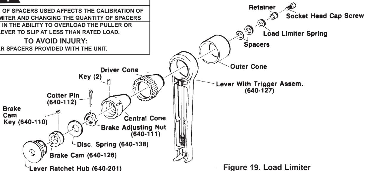
Figure 19. Load Limiter
