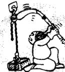
Never use an extension on the lever! You're dangerously overloading the Puller if you exceed the rated lever pull or if you have to use a lever extension to lift or pull a load.
