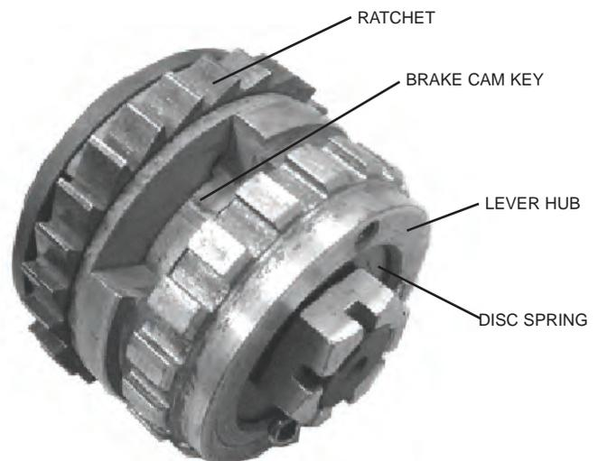
Figure 9. Brake Parts
