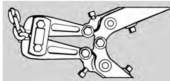
Figure 18. Cutting Chain with a Bolt Cutter
