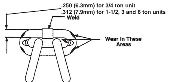
ring for this purpose). Compare these two measurements. If the stock diameter of the worn link is 0.010 inches (0.254 mm), or more, less than the stock diameter of the unworn link, the chain must be replaced.
