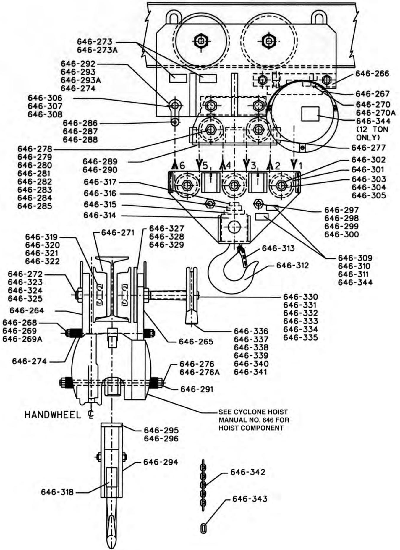
Note: When ordering parts, always furnish hoist model and serial number, motor horsepower, voltage, phase, frequency and rated capacity of hoist on which the parts are to be used.
