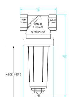
\*NOTE: ADDITIONAL CLEARANCE REQ'D FOR SCREEN REMOVAL: 5 3/4"
