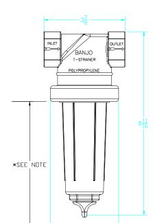
\*NOTE: ADDITIONAL CLEARANCE REQ'D FOR SCREEN REMOVAL: 5 3/4"
