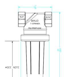
\*NOTE: ADDITIONAL CLEARANCE REQ'D FOR SCREEN REMOVAL: 5 3/4"
