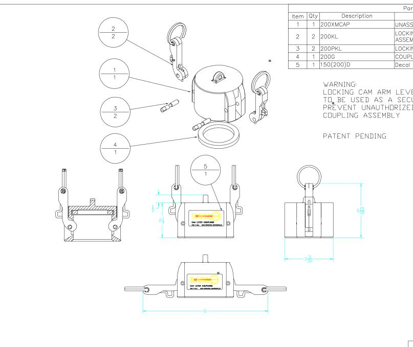
Parts list Note Material UNASSMBLD "CAP" CPLG POLYPROPYLENE LOCKING CAM ARM 316SS ASSEMBLY LOCKING CAM ARM PIN 316SS EPDM COUPLING GASKET
