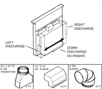
The system will operate most efficiently when the ductwork does not exceed 40 feet of equivalent duct. The chart above, shows equivalent feet of elbows and transitions. The number of feet of straight  $3\frac{1}{4}$ " x 10" or 6" duct plus the equivalent feet of elbows or transitions to be used should equal 40 feet or less.
