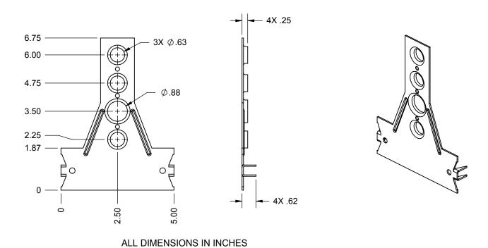
The HOLDRITE #109-N-6 is a Copper-Bonded™ steel bracket made to position 1/2" or 3/4" copper tube. Specifically designed to mount 1/2" stub-outs exactly 6" from the floor, with additional 5/8" holes at 2-1/4" and 4-3/4". There is a single 7/8" hole at the height of 3-1/2" for a hose bib, etc. This bracket also functions as a nail plate.
