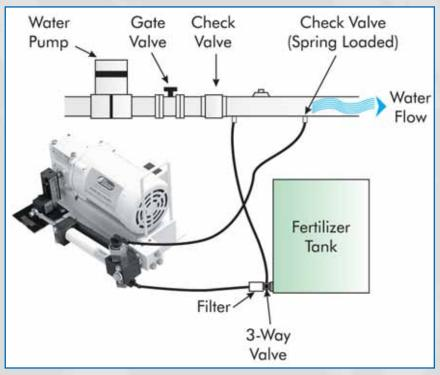
All CDS-John Blue Irrigation Pumps can be easily connected to your irrigation system and chemical tank to provide simple, reliable chemigation.
