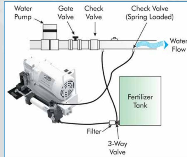
All CDS-John Blue Irrigation Pumps can be easily connected to your irrigation system and chemical tank to provide simple, reliable chemigation.
