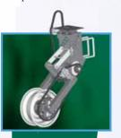
height. Ground Drive with pump mount - fixed height adjustn mechanism (10 positions), less tire and u-bolts.
