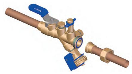
Under no circumstances should attempts be made to solder a Fig. \$1820 combination ball valve into the pipeline without first removing the union nut and solder connector from the body. This connector is soldered to the tube away from the valve. The warning label on the plastic bag should be read and understood.
