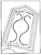
Apply a 1/8" bead of adhesive (supplied) as illustrated. Keep adhesive at least 1" away from factory applied pressure sensitive tape.
