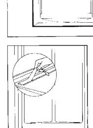
Remove backing from factory applied pressure sensitive tape.
