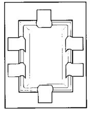
To assist in a secure fit, it is suggested that the Swanstone Recessed Accessory Shelf be held into place with either masking tape or hot glue. Tape the Recessed Accessory Shelf into position, or apply a dab of hot glue in each corner. This will hold the Swanstone Recessed Accessory Shelf in place until the silicone adhesive sets up. Allow 24 hours for drying.
