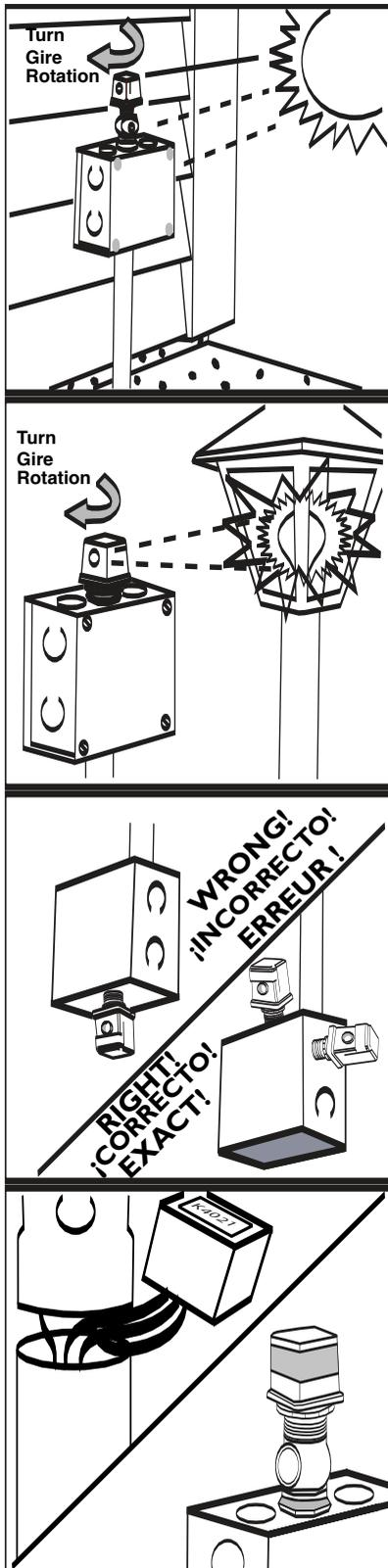
1. **Do not face the photocell into the midday sun.** If installed on the south side of a building, face east or west or point the photo control down toward the ground. The best direction to face the photo control is north.
