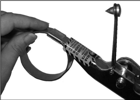
1. Tool is designed specifically for 3/8" and 5/8" center punch clamps only. Insert clamp in tool and then insert wrench assembly. If you prefer, install wrench assembly before clamp is inserted. Slot must be aligned with clamp tail.
