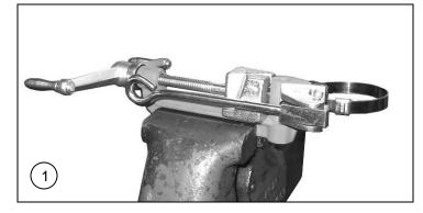
Place BAND-IT tool in vise. BAND-IT JR Adapter installs over nose of tool. Insert BAND-IT Junior or Junior SID Clamp in Tool and grip end of band by Band Gripper Lever contained in the slide block assembly of BAND-IT tool.
