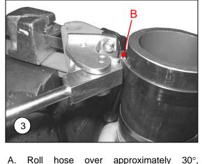
BACKING OFF TENSION HANDLE 1/2 to 1 turn only through course of rollover, depending on type and size of hose.
