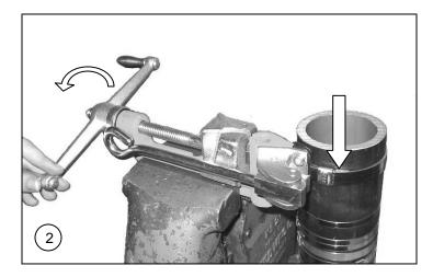
Install clamp over hose assembly. Tension clamp by turning the handle of BAND-IT Tool clockwise. To feel movement of band, place finger on BAND-IT BAND at buckle edge (shown by arrow) while tensioning with tool handle. When you no longer feel band moving through buckle, MAXIMUM PRESSURE HAS BEEN EXERTED BY BAND-IT BAND.
