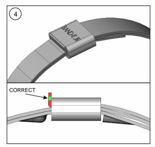
The finished BAND-IT JR. Smooth I.D. Clamp. Lip lock will be bent upward 90° and have a cut-off edge (shown in green) that is flush to the edge of the buckle. Edges shown in red are too high or too low and may result in lower lock strength or sharp edges.
