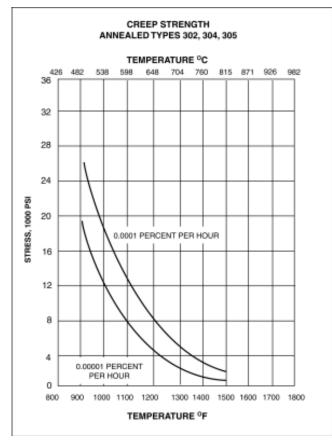
Data are typical and should not be construed as maximum or minimum values for specification or for final design. Data on any particular piece of material may vary from those shown herein.
