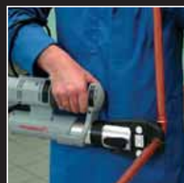
6. Manually open the jaws and locate over the fitting's bead, maintaining a 90° angle between jaws and tube. Start the operation. Ensure the tool cycles fully and the jaws close completely.
