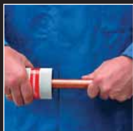
2. To prevent damage to the 'O' ring, IT IS ESSENTIAL THAT ALL BURRS ARE REMOVED AND THE OUTSIDE DIAMETER OF THE TUBE IS CORRECTLY CHAMFERED.
