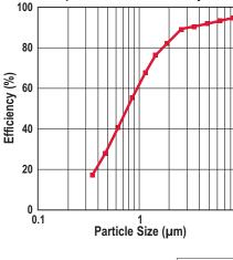
**Composite Minimum Efficiency Curve**
