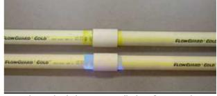
Any ultraviolet light source will identify joints that have been solvent cemented. The blue color ensures cement has been applied.
