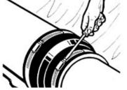
Tighten to 60 inch-lbs. torque.
