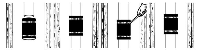
Loosen the stainless steel clamps. Do not remove clamps from coupling.
