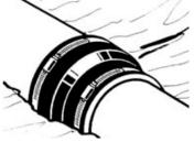
Pressure test before backfilling or concealing joint. Bed and backfill properly. (Max test pressure: 4.3 PSI or 29.6 KPA.)
