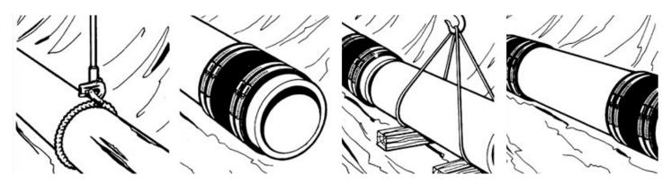
Fernco flexible couplings Remove pipe sections, can be used to couple pipe when there is a break, or an insertion is needed.
