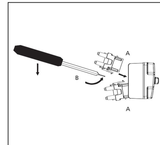
**4** Insertion Angle (A) / Securing the Connector (B)
