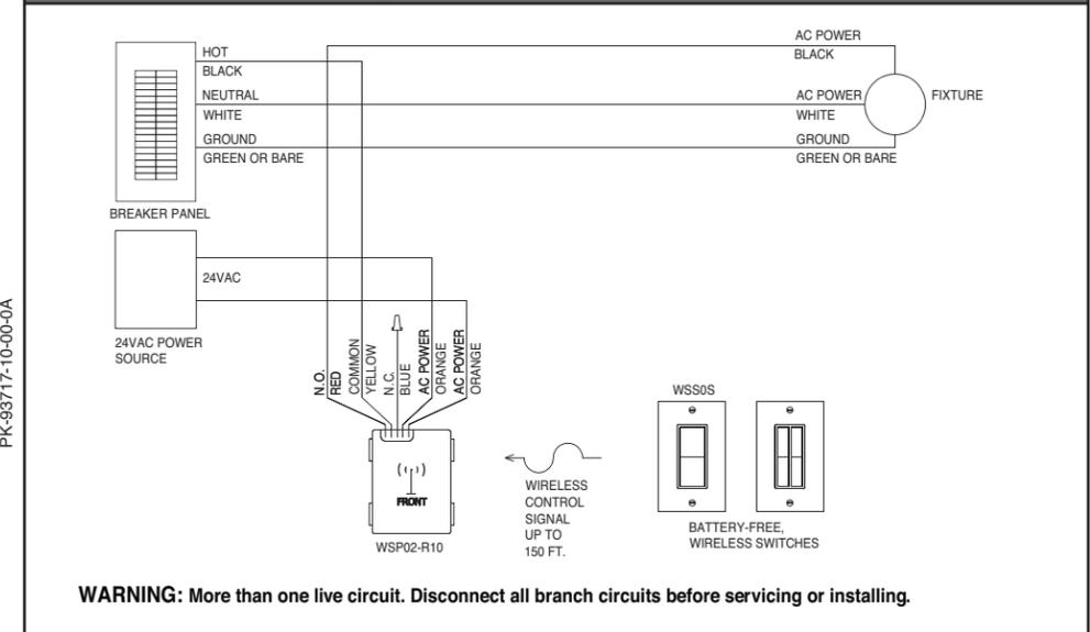
Figure F - Hardwired/Wireless Combo 4-Way Switch (1 hardwired 4-way, 1 hardwired 3-way, 1 wireless switch)
