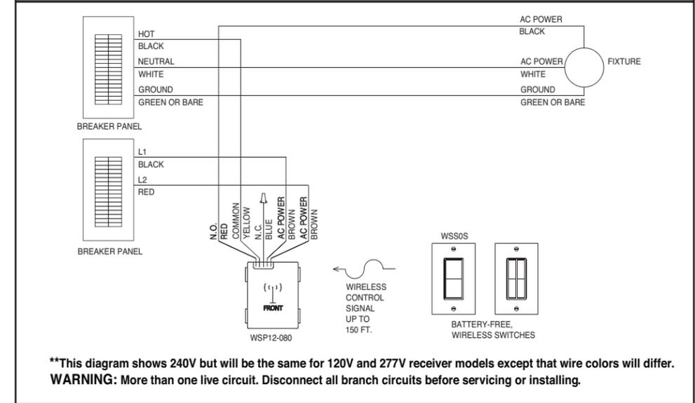
Figure E - Hardwired/Wireless Combo 3-Way Switch (1 hardwired 3-way switch, 1 wireless switch)\*
