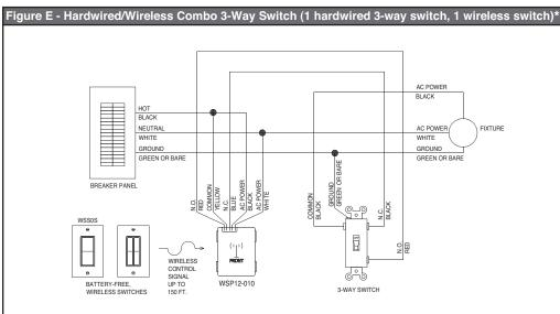
\*This diagram shows 120V but will be the same for 240V and 277V receiver models except that wire colors will differ. In this configuration, the maximum load is approximately 500W. See specifications for the N.C. relay contact.
