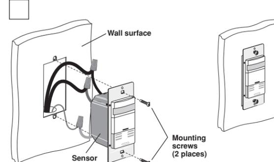
**NOTE:** Dress wires with a bend as shown in diagram to relieve stress when mounting device.
