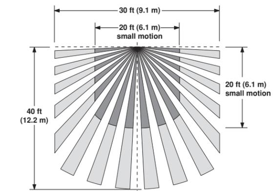
**Small Motion** = Dual Technology coverage. This also represents the maximum ultrasonic range coverage.
