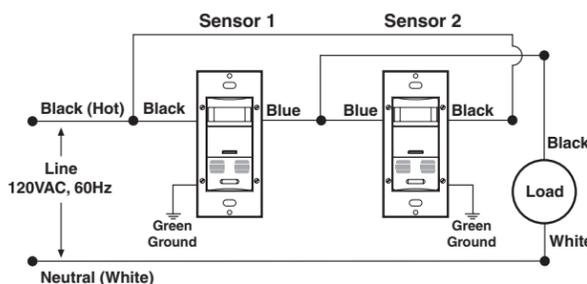
**NOTE:** Sensor 1 **must** be installed in a wall box that has both a LINE Hot and a Ground connection. Sensor 2 **must** be installed in a wall box that has both a Load and a Ground connection. If you are unsure about any part of these instructions, consult a qualified electrician.
