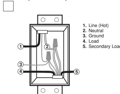
**Step 3** **Preparing and connecting wires:**
