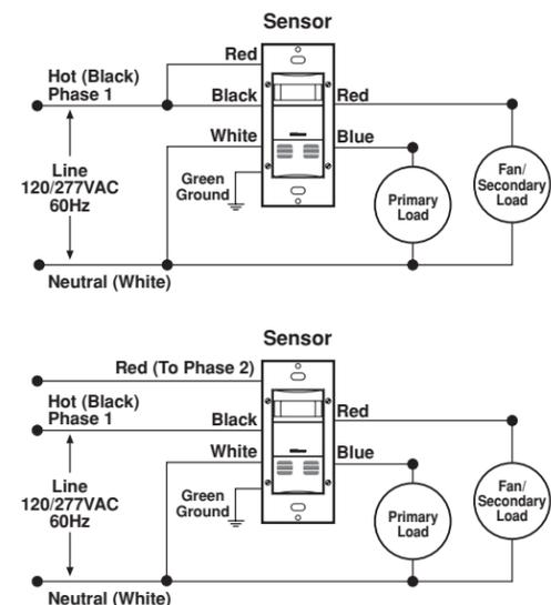
**Step 5** **Installing your Sensor - Two Location Wiring Application:**
