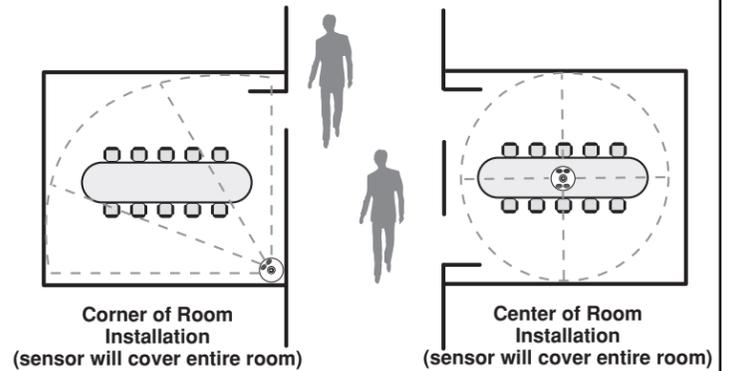
**NOTE:** When mounting device, do not point sensor openings towards the opening of a door or strong air currents.
