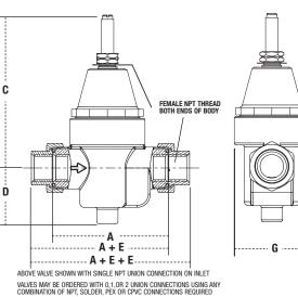
COMBINATION OF NPT, SOLDER, PEX OR CPVC CONNECTIONS REQUI "F" DIMENSIONS ARE APPROXIMATE ENGAGEMENT LENGTHS.
