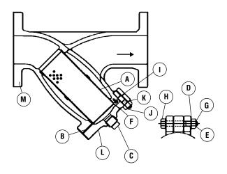
Screen AISI 304SS A. B. Cover Gasket Non-Asbestos C. D. Plug \*ASTM A47 Washer ASTM A6 E. Cotter Pin ASTM A112 F. \*ASTM A6 Plate G. **Bolt Nut** ASTM A6 H. Bolt ASTM A6 Set Screw ASTM B16 Cover Bolt Nut ASTM A6 J. K. Cover Bolt ASTM A6
