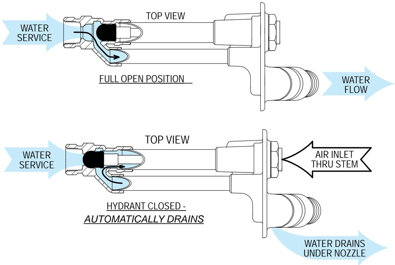
**NOTE: HYDRANT DRAINS AUTOMATICALLY WITH OR WITHOUT HOSE ATTACHED.**
