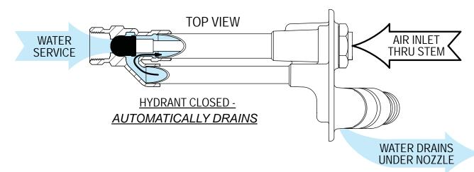
NOTE: HYDRANT DRAINS AUTOMATCALLY WITH OR WITHOUT HOSE ATTACHED. 04/10 Rev 2
