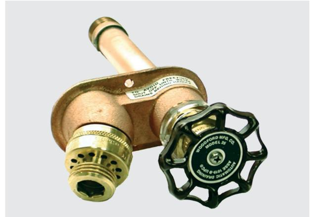
**NOTICE** - To close and drain, turn handle clockwise until seated and water drains out of the drain hole or faucet may freeze and burst. Vacuum Breaker replacement is recommended every 3-5 years.
