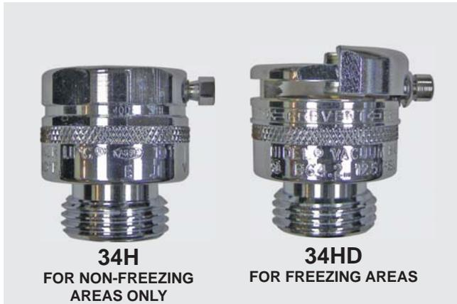
The NIDEL® Model 34H anti-siphon vacuum breaker is designed to protect hose connections from contamination where temperatures do not go below freezing. Uses include laundry tubs, utility sinks, boiler room hose bibbs and outside hose bibbs in non-freezing areas.
