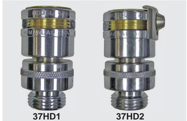
The NIDEL® Model 37HD1 / 37HD2 hose connection backflow preventers are designed to protect hose connections from backflow contamination in freezing and non-freezing conditions. Manual draining is required and provides easy, sure drainage during freezing weather. Uses include outside hose bibbs, wash racks, dairy barns and swimming pool areas.
