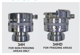
The NIDEL® Model 34H anti-siphon vacuum breaker is designed to protect hose connections from contamination where temperatures <u>do not go below freezing.</u> Uses include laundry tubs, utility sinks, boiler room hose bibbs and outside hose bibbs in non-freezing areas.
