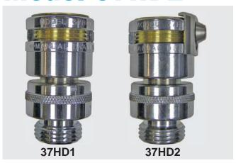
The NIDEL® Model 37HD1 / 37HD2 hose connection backflow preventers are designed to protect hose connections from backflow contamination in freezing and non-freezing conditions. Manual draining is required and provides easy, sure drainage during freezing weather. Uses include outside hose bibbs, wash racks, dairy barns and swimming pool areas.
